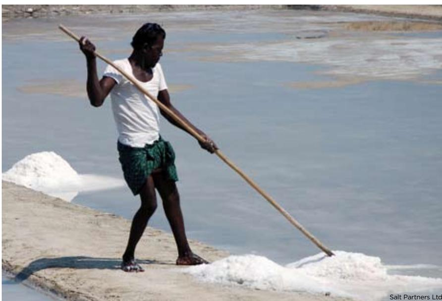
In Tuticorin, India, perhaps the simplest method of salt harvesting with wooden tools from shallow earthen ponds is being practised. A similar salt harvesting method is still being used in small saltworks all around the world.
