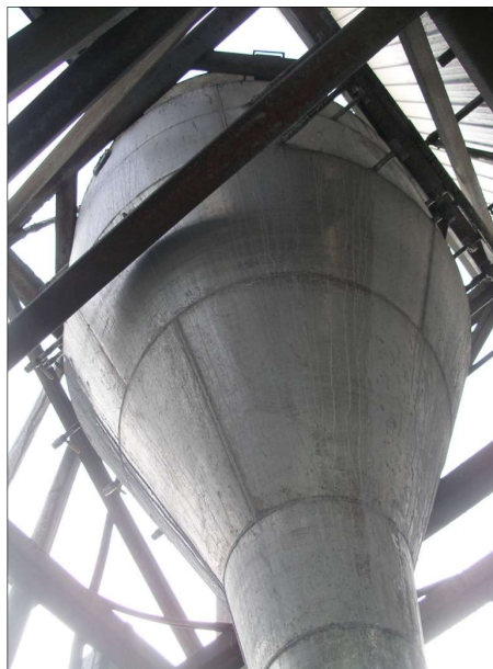
Salt Partners HYDREX-4 hydroextractor for slag desalting, co-invented by Vladimir M. Sedivy, Patent No. CH690840
