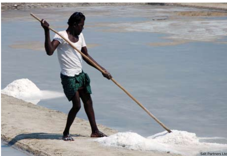
In Tuticorin, India, perhaps the simplest method of salt harvesting with wooden tools from shallow earthen ponds is being practised. A similar salt harvesting method is still being used in small saltworks all around the world.
