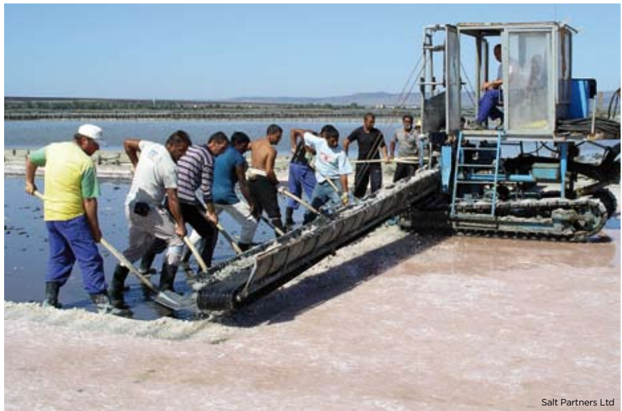
A team of men pick the salt from the mud floor of a crystalliser by shovels to suspended belt conveyors, which transport the salt to a slurring vessel located on a tractor. Salt is mixed with brine and pumped to a mobile washplant located at the side of the crystallising pond.
