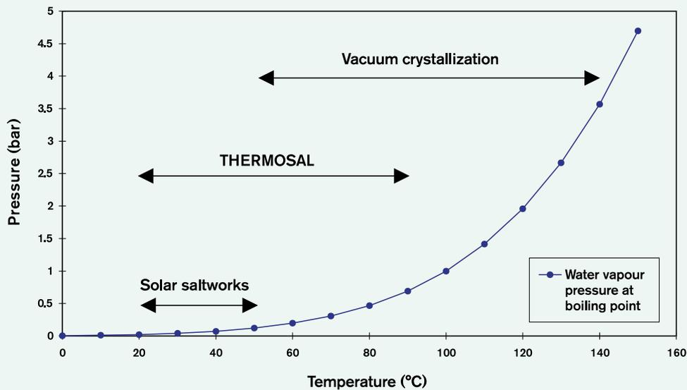
Figure 2. Operating ranges of salt production processes
