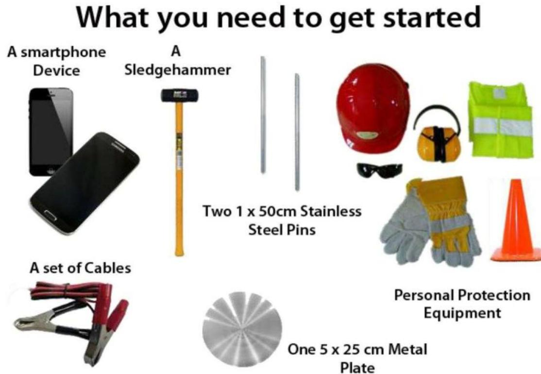
For our electro-seismics mapping work, we used the following equipment:
