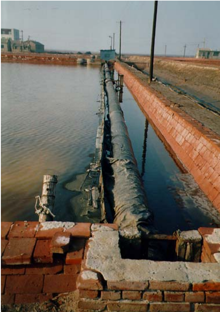
Chinese solar salt crystallising pond with rain protection foil
