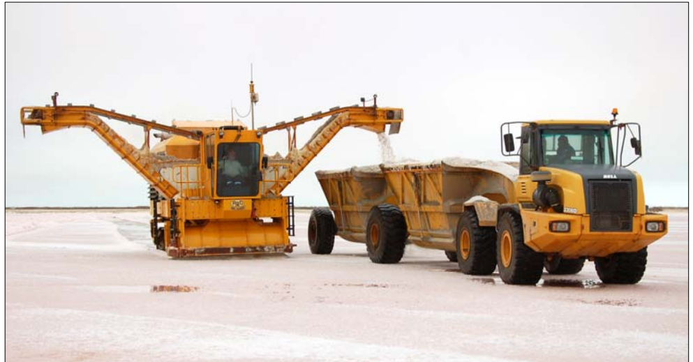
Durrant 7160-95 salt harvester in operation at Walvis Bay in Namibia
