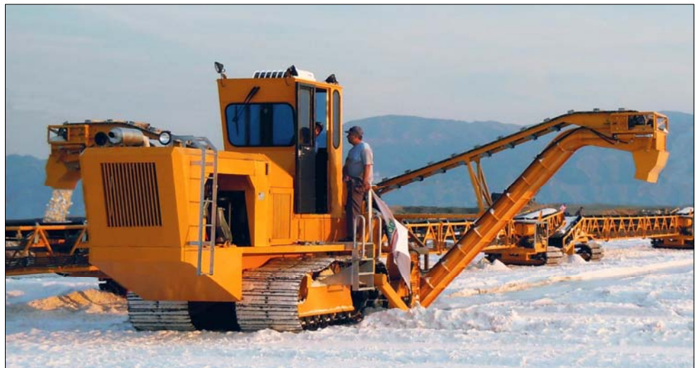
Durrant 566-70 salt harvester in operation with mobile belt conveyors
