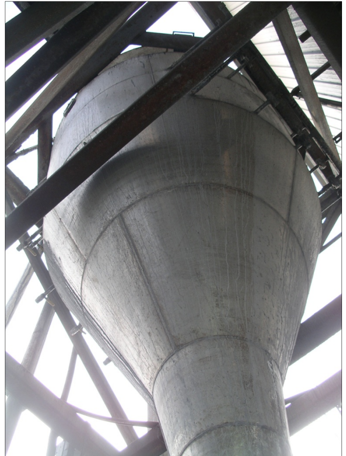
Salt Partners HYDREX-4 hydroextractor for slag desalting co-invented by Vladimir M. Sedivy, CH Patent No. 690840
