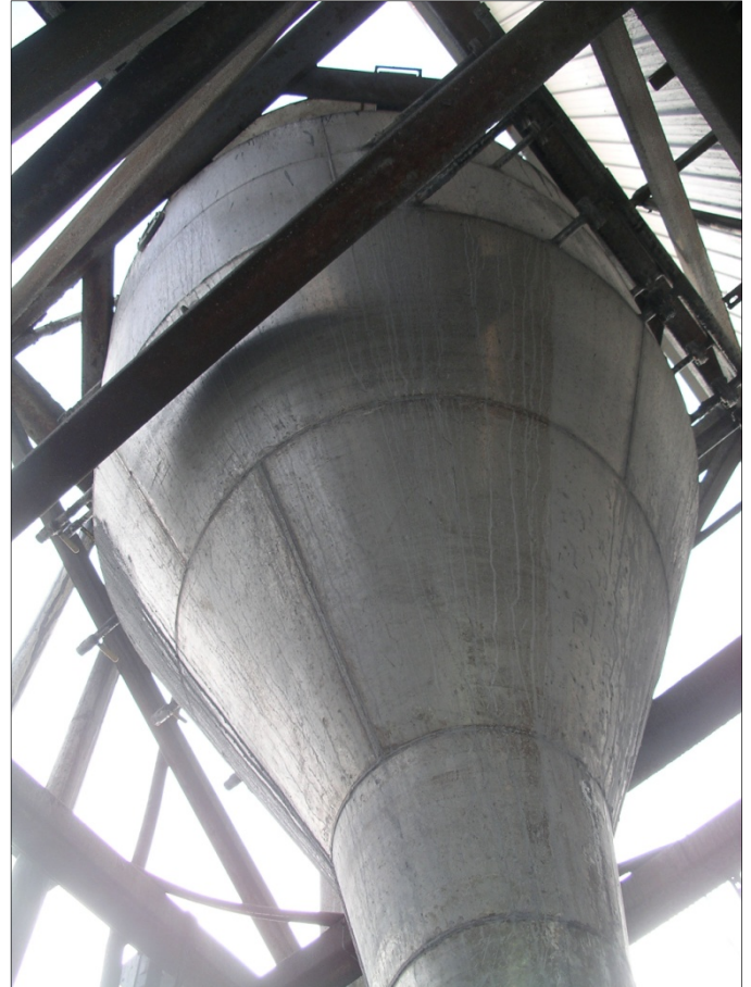
Salt Partners HYDREX-4 hydroextractor for slag desalting co-invented by Vladimir M. Sedivy, Patent No. CH690840
